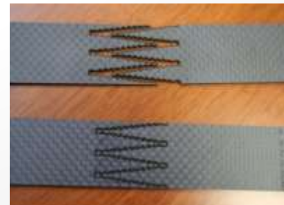
モザイク突合せ継手のレーザ加工 Laser cutting and joining of mosaic butt joint
